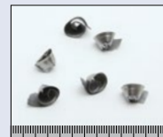
Ø20 hole processing (non-step drilling)
